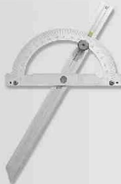
*Goniometer with precision sliding rod. Made from galvanically treated, anti-corrosion steel. Angle capacity 10-170° with 1° graduations. Etched, easy to read, long-lasting. With double base.*
