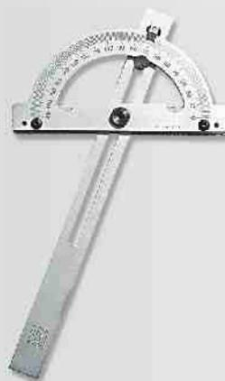
*Adjustable goniometer. Made from galvanically treated, anti-corrosion steel. Angle capacity 10-170° with 1° graduations. Etched, easy to read, long-lasting. With double base.*
