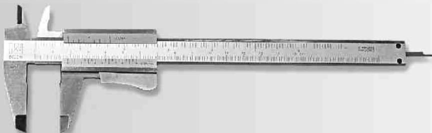
*Caliper in stainless steel with assembled slider. Satin-chromed precision scale, easy to read and long-lasting. Raised slider for easy movement. **Slider locking button**. Five functions. Manufactured as per DIN 862. Supplied in sheath.*
