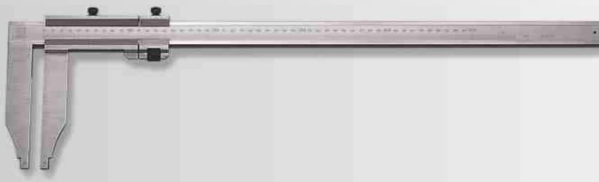
*Monoblock caliper in hardened stainless steel. Satin-chromed readout scale. Etched, precision graduation, easy to read and long-lasting. Raised slider for easy movement. Slider locking screw with micrometric adjustment and lapped contact surfaces.*
