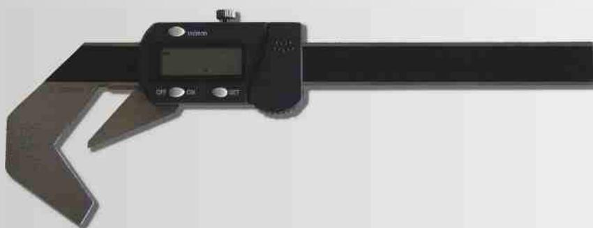
*Monoblock digital caliper in hardened stainless steel. Suitable for measuring the diameter of side-mills. With screw clamp. Serial number. Manufactured as per DIN 862. Supplied in sheath.*
