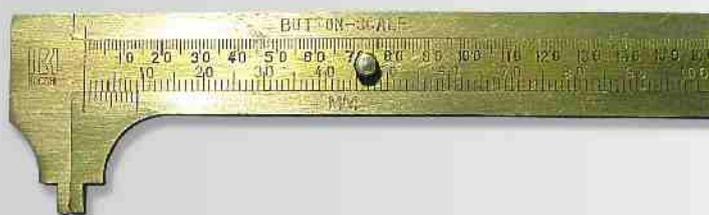
**Brass caliper** with division in mm and special division for buttons.
