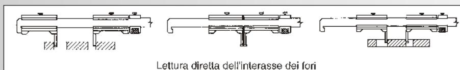
*Monoblock caliper in hardened stainless steel. Satin-chromed readout scale. Etched, precision graduation, easy to read and long-lasting. Raised slider for easy movement. Suitable for measuring spacing between holes, with 25 mm long stylus points. Slider locking screw with micrometric adjustment. Slide stop at beam end. Serial number.*
