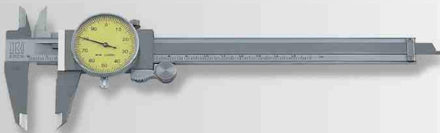
*Caliper in hardened stainless steel with precision dial-gauge. Satin-chromed readout scale. Slider locking screw with adjustment wheel. Steel rack protected from dust. Revolving dial-face with lock. Five functions operation. Serial number.*
