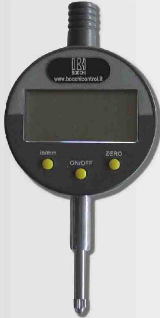
**Workshop digital indicator.** Digital display LCD, height of digits 8,5 mm. Mm/inch conversion. Setting to zero in any position. Measuring pin in hardened and ground stainless steel. Clamping: Stem  $\varnothing 8 - h6$  in hardened and ground stainless steel. Interchangeable contact point M2,5. Powered with one battery. With serial number. Manufactured as per internal rule. Supplied in case.
