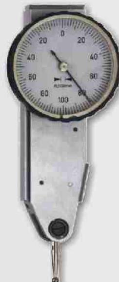
**Test indicator.** Ruby-mounted gear movements give maximum precision but the test indicator is also shockproof. Automatic inversion of the direction of measurement without a switch to anticlockwise direction of the indicator. Supplied with three guides for attachment to comparator holders for greater versatility. Complete with Ø 2 mm ball probe tip and Ø 8 mm connector. Manufactured as per DIN 2270 form B. Supplied in case.
