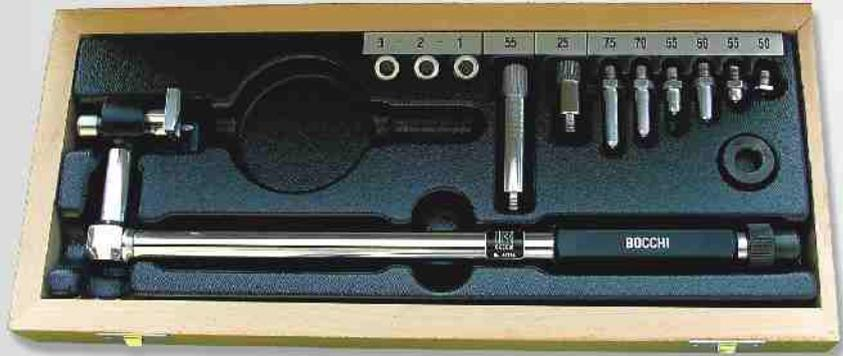
**Right-angled bore gauges** suitable for measuring cylinders and bearing seatings square to the axis of the instrument. Contact points in hardened steel. Body in chromed steel with heat-insulated grip. Manufactured as per DIN 878. Supplied in case without dial indicator. **Art. 5273 version with carbide contact points.**
