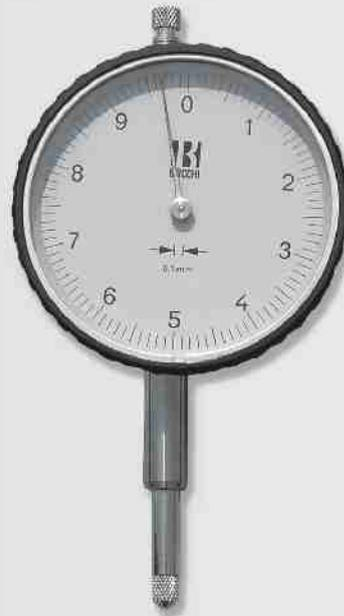
*Shockproof, decimal dial indicator with advanced technology transmission mechanism. Shocks received by the probe are not transmitted to the internal mechanisms so that precision remains constant. Rotating bezel with tolerance markers. Manufactured as per DIN 878. Supplied in case.*
