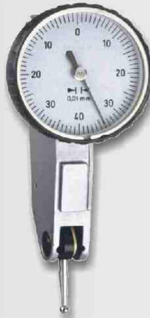
**Test indicator.** Ruby-mounted gear movements give maximum precision but the test indicator is also shockproof. Automatic inversion of the direction of measurement without a switch to anticlockwise direction of the indicator. Supplied with three guides for attachment to comparator holders for greater versatility. Complete with Ø 2 mm ball probe tip and Ø 8 mm connector. Manufactured as per DIN 2270 form A. Supplied in case. .
