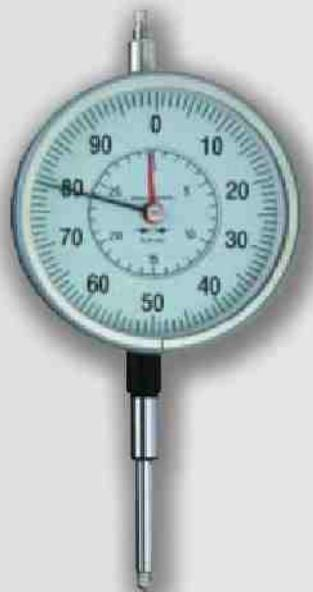
*Shockproof dial indicator with big dial. Robust metal housing and construction, assure the accuracy on all range. Insulated internal mechanisms to avoid shocks. The bezel together with the outer dial can be rotated to set zero in any position. Manufactured as per DIN 878.*
