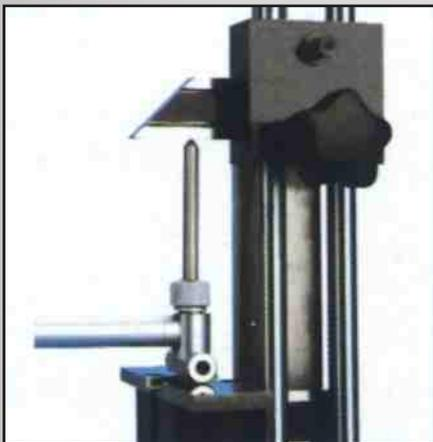
***Bore gauge setting instrument**, this instrument offers you the best way to accuracy zero-set your bore gauges and internal micrometers at two contacts. Gauge blocks are used to set the exact reference value. Measuring range 18-400 mm. The setting instrument consists of a stand with double guidance and flat measuring jaw, a couple of hardened steel contacts and one support for bore gauges.*
