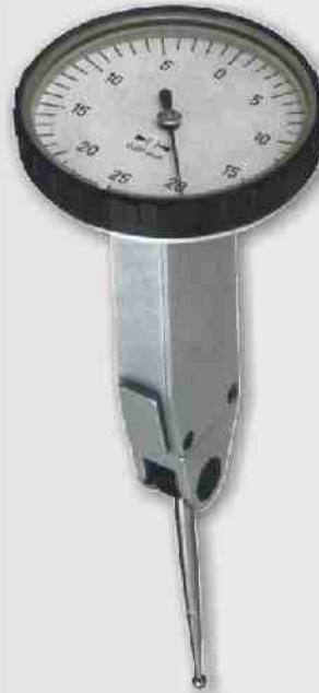
**Test indicator.** Ruby-mounted gear movements give maximum precision but the test indicator is also shockproof. Automatic inversion of the direction of measurement without a switch to anticlockwise direction of the indicator. Supplied with three guides for attachment to comparator holders for greater versatility. Complete with Ø 2 mm ball probe tip and Ø 8 mm connector. Manufactured as per DIN 2270 form C. Supplied in case. .
