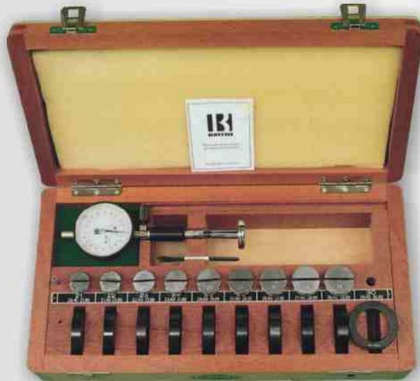
**Comparators suitable for checking cylindrical bores** to determine their diameter and errors of shape. The standard tracer points are fitted with convex surfaces in hardened chrome to facilitate insertion into the bore. Any grooves or recesses in the bore will not hamper measurement. Axial centering is achieved by moving the bore gauge from side to side. Supplied in case with setting rings but without dial indicator. Extension can be mounted to increase the depth. Manufactured as per DIN 878.
